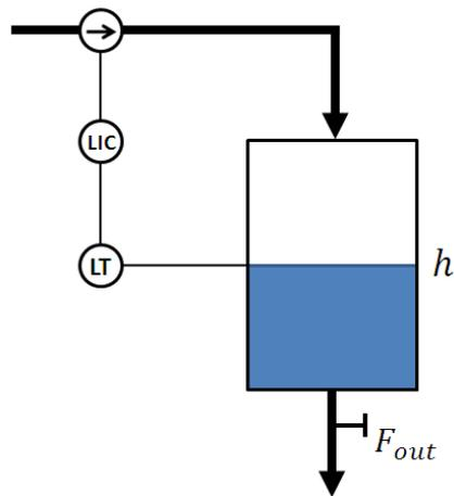
The purpose is to control the level in the water tank. In order to communicate with the physical process, we use a NI USB-6008 DAQ device:
